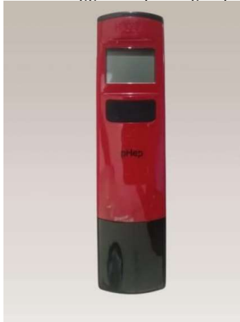
Gambar 1. pH Air HANNA INSTRUMENT HI98107
